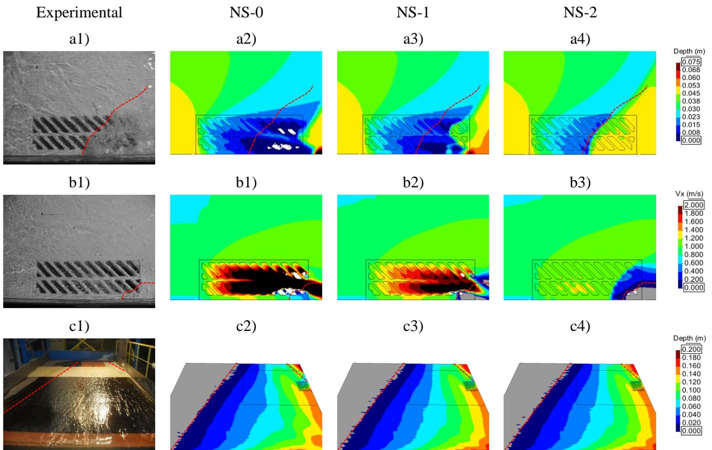
**Figure 4:** Flow patterns: hydraulic jump (a); recirculation area (b); cross waves (c). Flume configuration [discharge and longitudinal-transverse slopes]: 200 l/s and 4 %-0 % (a); 100 l/s and 2 %-0.5 % (b); 100 l/s and 4 %-10 % (c). Flow patterns are highlighted in red-dashed line.
