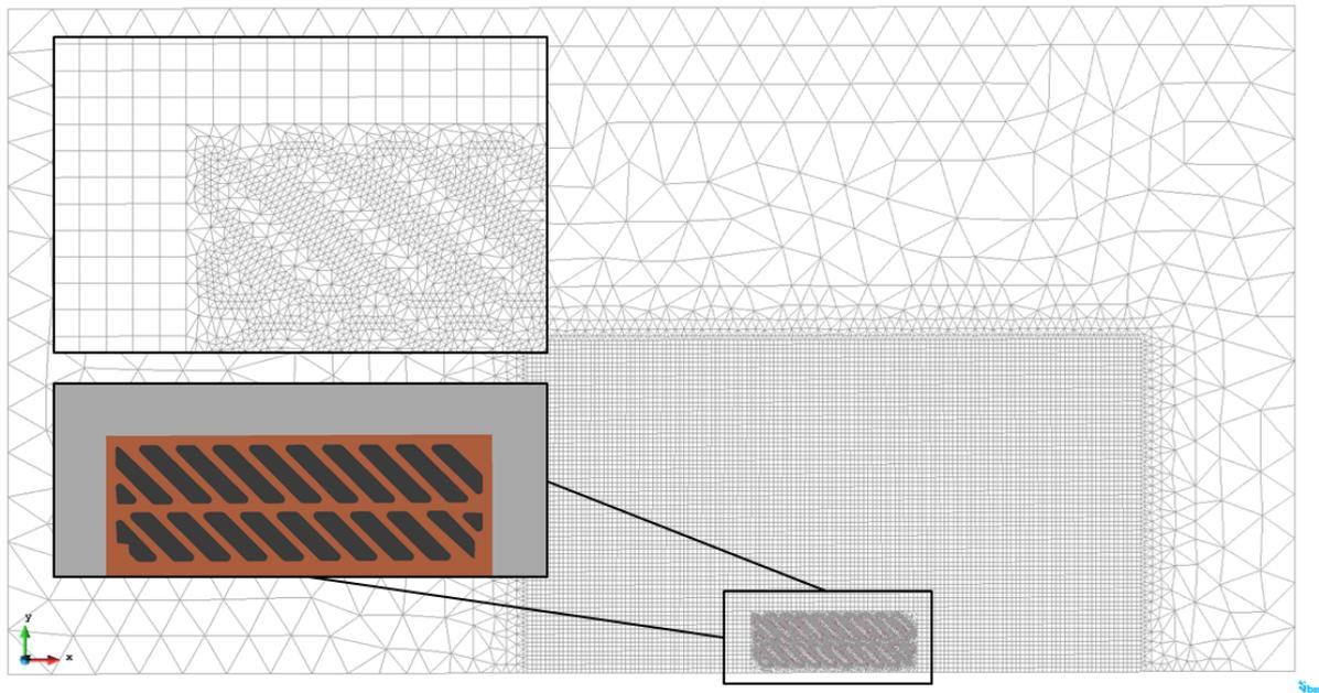
**Figure 3:** Flume discretization and mesh accuracy for gutter inlet. The different parts of the model were coloured (grey: flume platform; orange: inlet grate; black: inlet holes).
