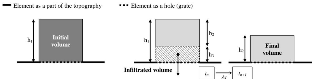
Figure 2: Description of the infiltration process in a hydraulic model.
